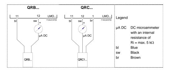
As an alternative to detector current measurement, the diagnostic tool OCI400 / ACS400 can be used. In that case, the DC microammeter is not required.
