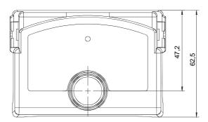
LMO... with extension of lockout reset button AGK20...
