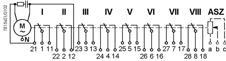
Diagram shows the maximum number of switches (2 end and 6 auxiliary switches). On versions with fewer than 6 auxiliary switches, the higher numbers are not used. For example, the actuator version with 2 end and 2 auxiliary switches does not use switches V, VI, VII and VIII.
