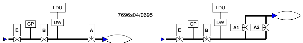
Plants without vent pipe to atmosphere
