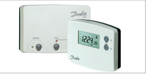
The TP5001 is a microprocessor based programmable room thermostat with many advanced features. The range includes battery and 230 volt powered hard-wired models and battery powered wireless versions. All models in the range utilise an advanced PI algorithm to provide close and accurate temperature control to reduce energy waste and ensure comfort under all load conditions.
