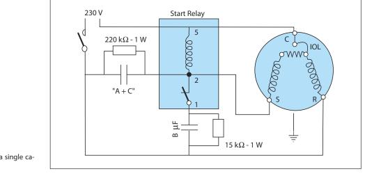
Motor protector A + C Run capacitors В Start capacitor С Common
