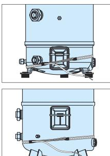
Under extreme conditions such as low ambient temperature at -15°C or lower a belt type crankcase heater could be used in addition to the PTC heater, although this is not a preferred solution for 1 and 2 cylinder compressors. The belt crankcase heater must be positioned on the compressor shell as close as possible to the oil sump to ensure good heat transfer to the oil. The below illustrated mounting positions are recommended:
