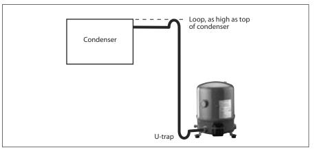
In most installations the initial compressor oil charge will be sufficient. In installations with line runs exceeding 20 m, or with many oil traps or an oil separator, additional oil may be required. In installations with the risk of slow
